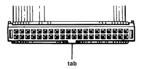
Pull the cable over toward the socket and fold it to align the connector with the socket. Make sure the side of the connector with the tab lines up with the side of the socket with the notch. Then line up the holes over all of the pins and push in the connector.
